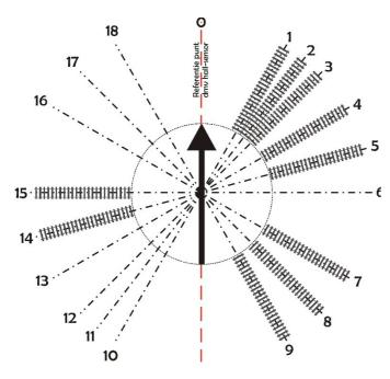
Train controller software should be set in a way that turntable is defined as Märklin Turntable. This implies that rail positions 1..9 are used. Positions 10..18 are assumed to be 'the opposite side'.
