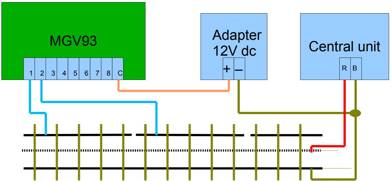
In this example, the standard Maerklin contact system is used on two contact rails.
